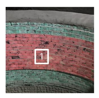
As per the SOP of JSW Dolvi, rings in Steel Ladle are substituted until a LOT of 110mm minimum is found.
